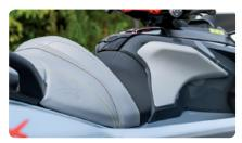
**Ergolock™ System** A narrow seat profile with deep knee pockets lets riders sit naturally and use the lower body to hold onto the machine for more control.
